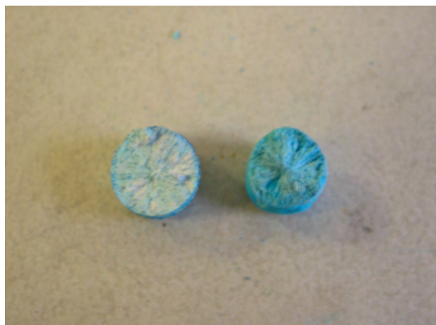
Figure 5.12 Optical image showing cross sections of aligned porous MOF composites prepared using DMSO. The loadings between polyTEGDMA scaffolds (left) are compared with \text{NH}_2 functionalized scaffolds (right). Scaffolds were prepared using 1:10 monomer/dioxane (v/v) solutions. Monoliths are 7 mm in diameter.
