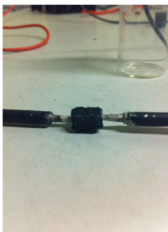
Figure 2.5 Image of voltmeters attached to porous polymer sample by conductive silver adhesive.
