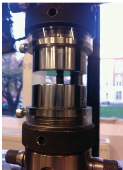
Figure 2.6 Image of porous polymer placed between two loading cells for compression testing.
