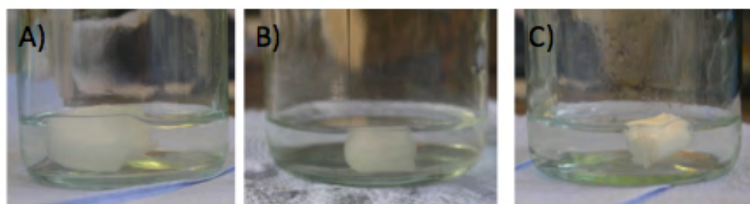
Figure 4.6 Images of polyDMAEMA (1:5 DMAEMA to dioxane (v/v), 3% EGDMA) placed in A) 1 M HCl aqueous solution, B) distilled water and C) 1 M NaOH aqueous solution.
