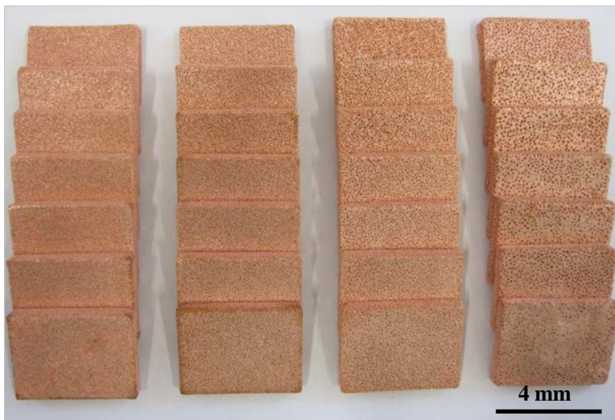
Figure 3.6 Typical porous copper samples assembly after sintering.
