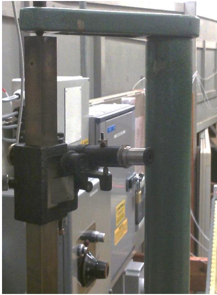
Figure 3-20 - Cathetometer (travelling microscope) used to measure hot-wire wall-normal proximity
