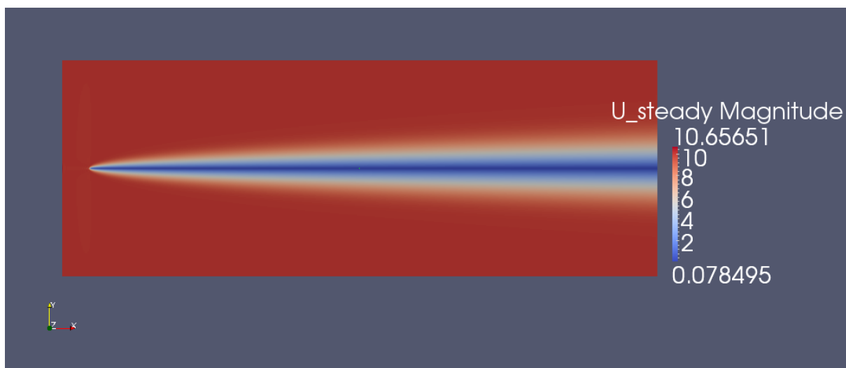
Figure 5-3 - Contour plot of velocity magnitude for steady ZPG flow (stretched in normal direction) [m/s]
