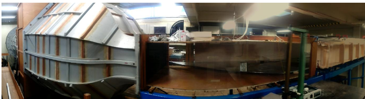
Figure 3-2 - Panoramic view of the tunnel, measuring and ancillary equipment with the positive pressure gradient section fitted
