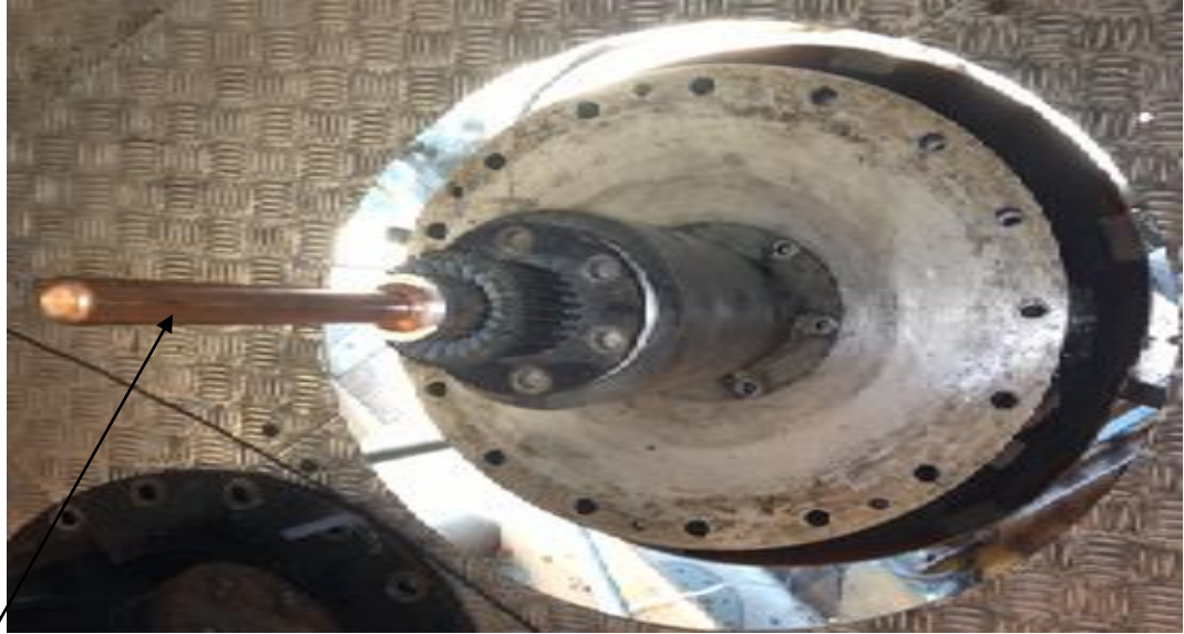
Figure 3.10 shows the moving contact sub-assembly Poker (i.e., moving contact)
