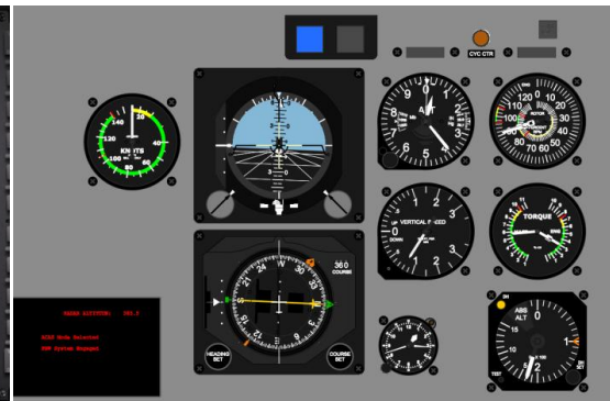
Figure 3-9 - Bell 412 Instrument Panel Generated in VAPS XT
