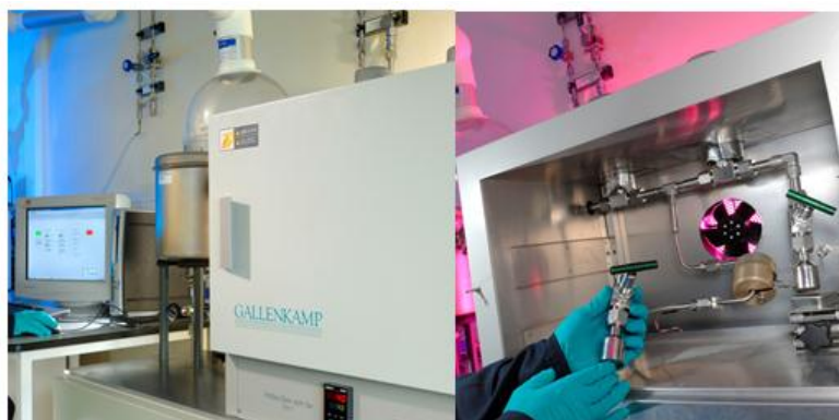
Figure 48 The vapour pressure system at SAFC Hitech.
