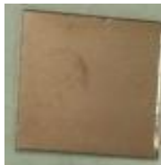
Figure 91 Copper film deposited from Cu(hfac)(COD) on glass at 250°C with no co-reagent.
