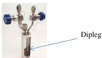
Figure 18 A stainless steel bubbler .
