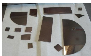
Figure 97 Photographs showing copper deposition on glass, silicon and TiN substrates. 10,000cycles, 100°C, H plasma, cooled under vacuum.
