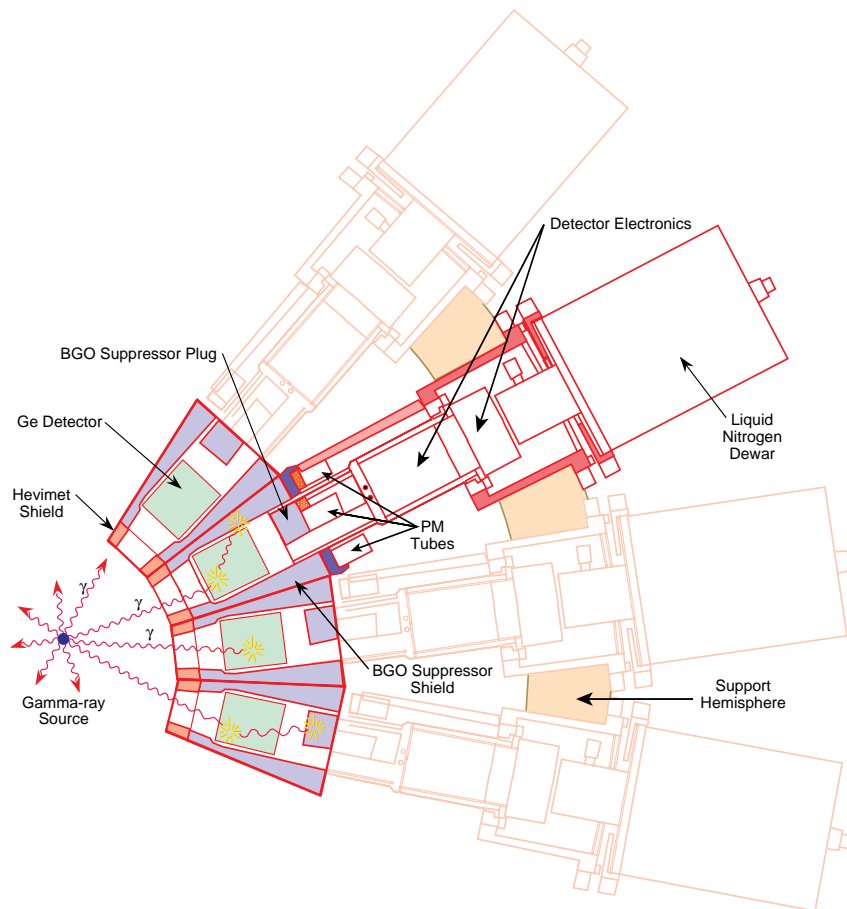
FIGURE 3.2: Schematic of a HPGe detector in the Gammasphere array. The principle of Compton suppression is also illustrated: The upper and lower gamma rays are scattered out of the HPGe crystal, but are detected by the BGO suppression shields, meaning their energies can be vetoed. Reprinted from Ref. [47].
