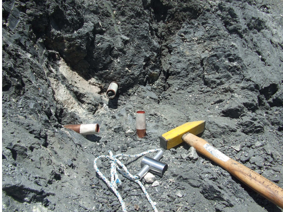
Figure 4.6: Photo showing collection of gouge samples. Copper tubes were hammered into the fault gouge. They were then removed and the ends of the tubes were secured with glue.
