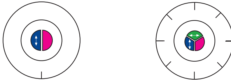
Figure 4.4: Schematic diagram showing the geometry of the piezoelectric crystals in the sample assemblies. The two pulsing crystals are shown to the left, and the three receiving crystals to the right. The crystals shown in pink pulse waves with a P-wave polarisation i.e. polarisation direction parallel to the direction of travel. Those shown in blue and green pulse waves with S-wave polarisations. The polarisation directions are indicated by the arrows.
