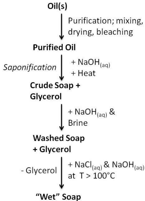
Figure 2-26 Flow diagram of generic industrial saponification process.
