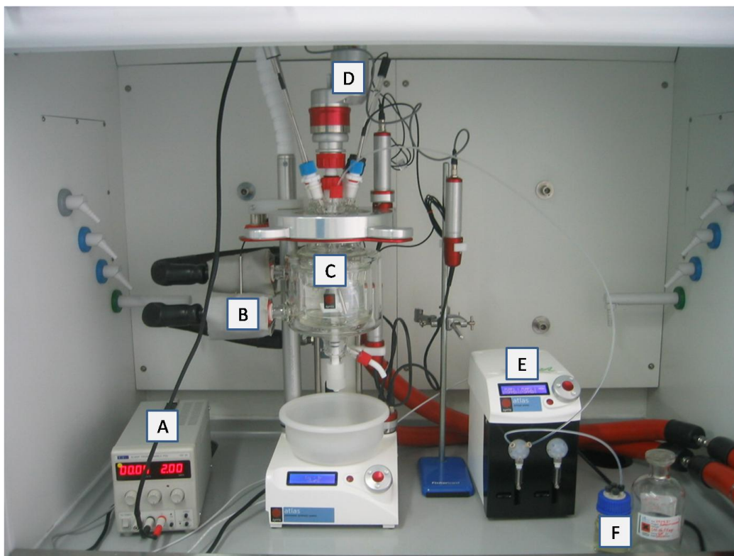
Figure 9-1 Atlas Potassium Calorimetry Reactor equipment setup. A) Power controller for power compensation reactor heater, B) Jacket-In temperature probe ( T_j ), C) Vacuum triple jacketed 500mL reactor containing 400mL of [1M] \text{NaOH}_{(\text{aq})} with pH, temperature ( T_r ) and turbidity probes, D) Controlled overhead mechanical stirrer, E) Reagent feed delivered by controlled Atlas syringe pump, F) Feed reservoir of 100mL sunflower oil [8].
