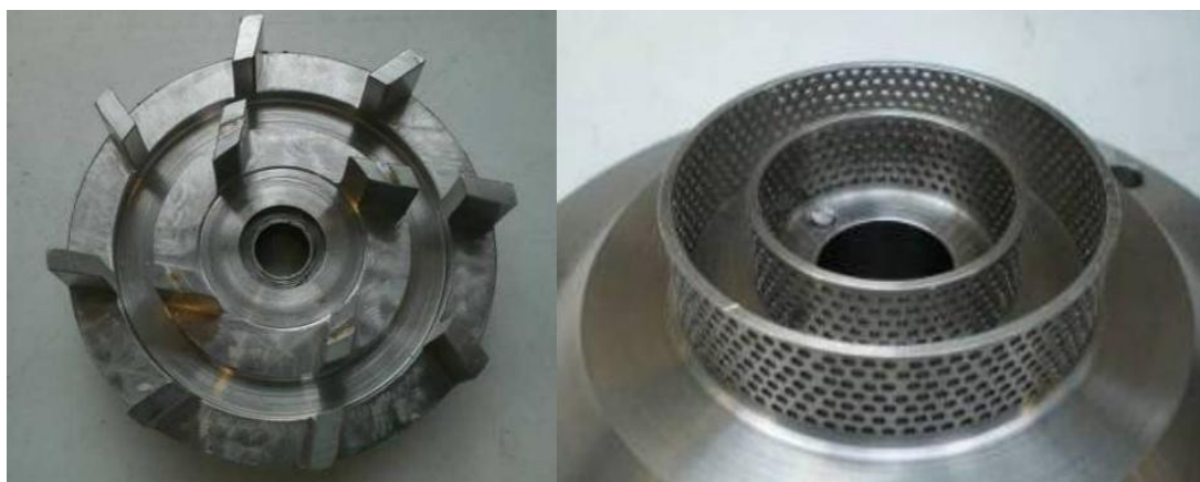
Figure 5-2 Silverson 150/250 MS rotor (left) and stator (right) (Hall et al., 2011)
