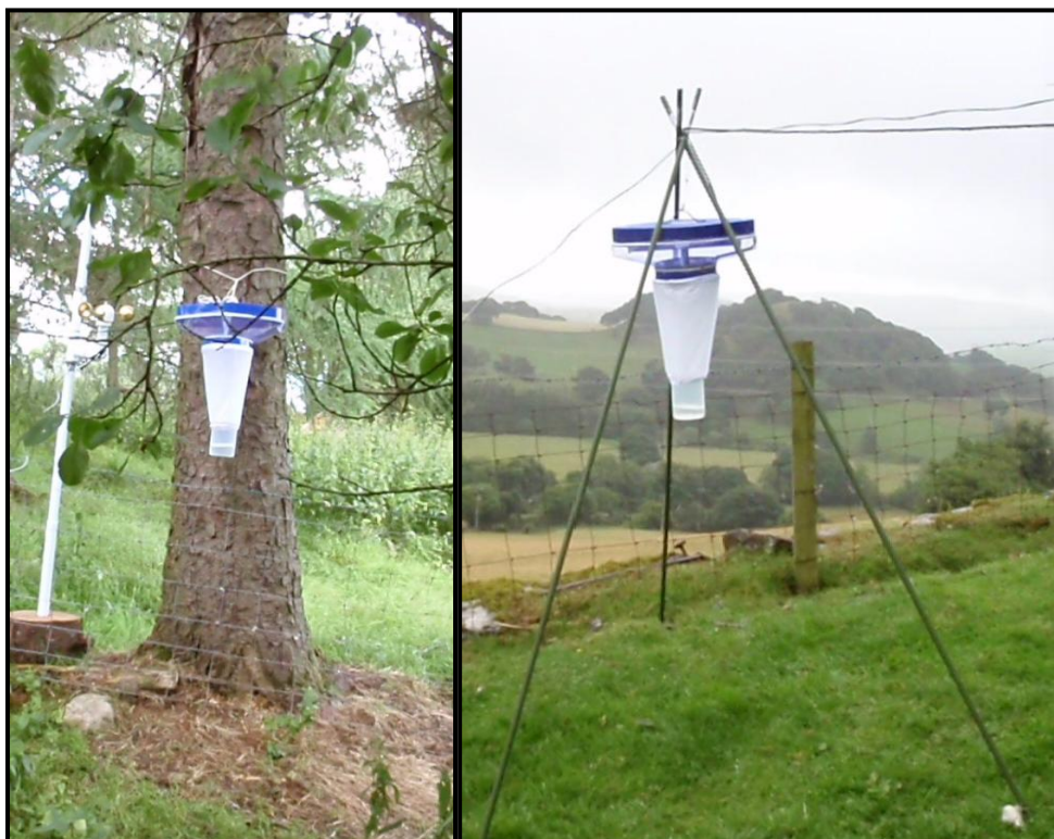
Figure 2.4 Onderstepoort Veterinary Institute (OVI) 8W UV light trap, hung from a tree (left) and a tripod (right).
