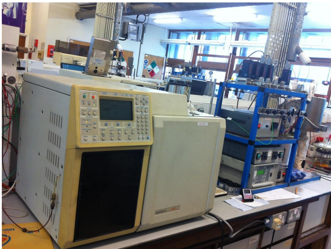
Figure 2.10 Varian 3800 gas chromatograph with Varian Star Software equipped with ZB-WAX capillary column and a flame ionization detector.
