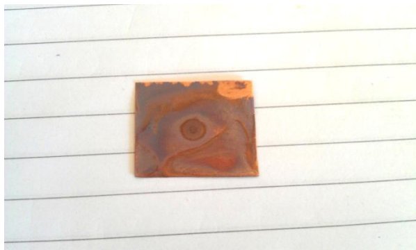
Figure 51: First sample after concentrated HNO 3 dip, rinsing in water and ethanol and several hours left in air.
