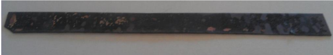
Figure 74: Photograph of sample surface (compression) after annealing while coiled, flattening then oxidising in an ambient atmosphere at 500°C for 150 minutes. The end in the left of the image has undergone the most deformation. Visual inspection shows a less reflective surface at the less deformed end indicating a higher density of nanowires.
