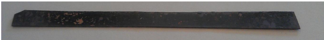
Figure 75: Reverse surface (tension) of same sample as shown in Figure 74. Visual inspection shows a small area of low reflectivity (from around 1-3cm along from the left hand edge).
