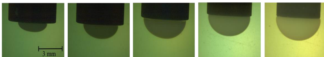
Figure 3 Photographs of gels of BrNapFV grown on glassy carbon electrodes at different currents: (from left to right) 5 \mu\text{A} , 20 \mu\text{A} , 40 \mu\text{A} , 60 \mu\text{A} , 80 \mu\text{A} . All gels were grown for 1000 s. The scale bar applies to all images shown
