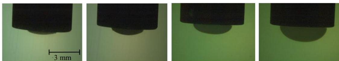
Figure 5 Photographs of gels of 2NapAA grown on glassy carbon electrodes at different currents: (from left to right) 20 \mu\text{A} , 40 \mu\text{A} , 60 \mu\text{A} , 80 \mu\text{A} . All gels were grown for 1000 s. The scale bar applies to all images shown
