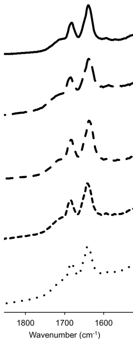
Figure 14 Partial FT-IR spectra of FmocFF gel samples (from top to bottom) before washing, after 1, 2, 3 and 4 washings, respectively
