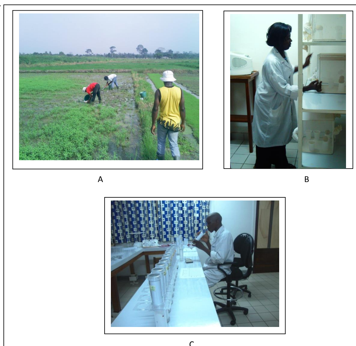
Figure 2.1: Illustration of field collections and susceptibility assays showing (A) Larval collection in Tiassalé rice field, (B) Larval-rearing and (C) Exposure to insecticides using WHO bioassay tubes
