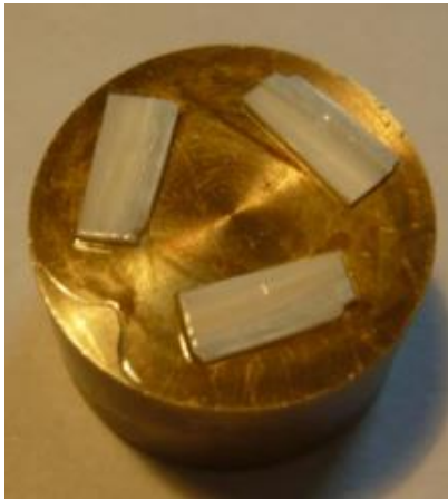
Figure 3. 7- Diamond disk to hand polish the samples mounted on brass anvils
