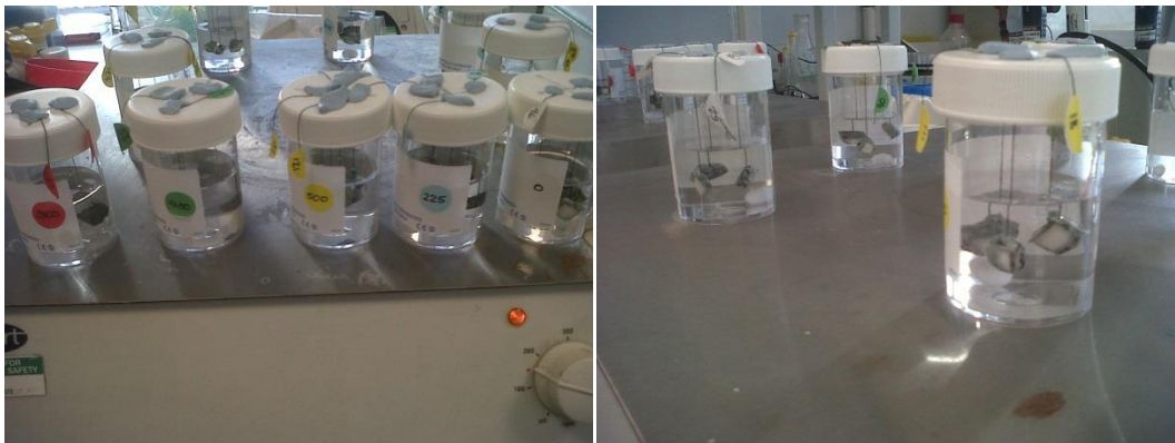
Figure 3. 12 – samples suspended in solutions per group with magnetic flea in each pot and placed on a stuart stirrer.
