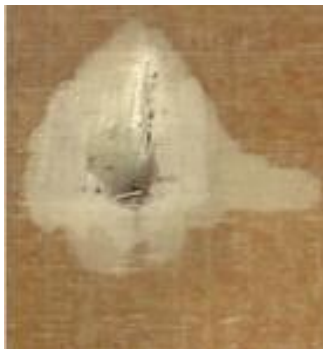
Figure 4.67 Photographs showing the top skin of the linear PVC (R63.140) sandwich structures following a 20 J impact at (a) 0° ; (b) 10° ; (c) 20° inclination angles.
