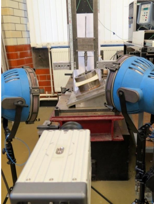
Figure 3.6 The Instrumented drop-weight impact test set-up for oblique impact testing ( 20^\circ inclination).
