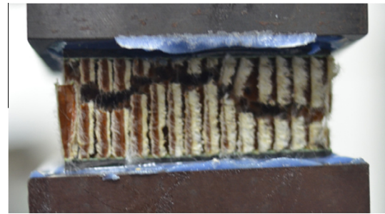
Fig. 9. Failure mode of the tensile test.
