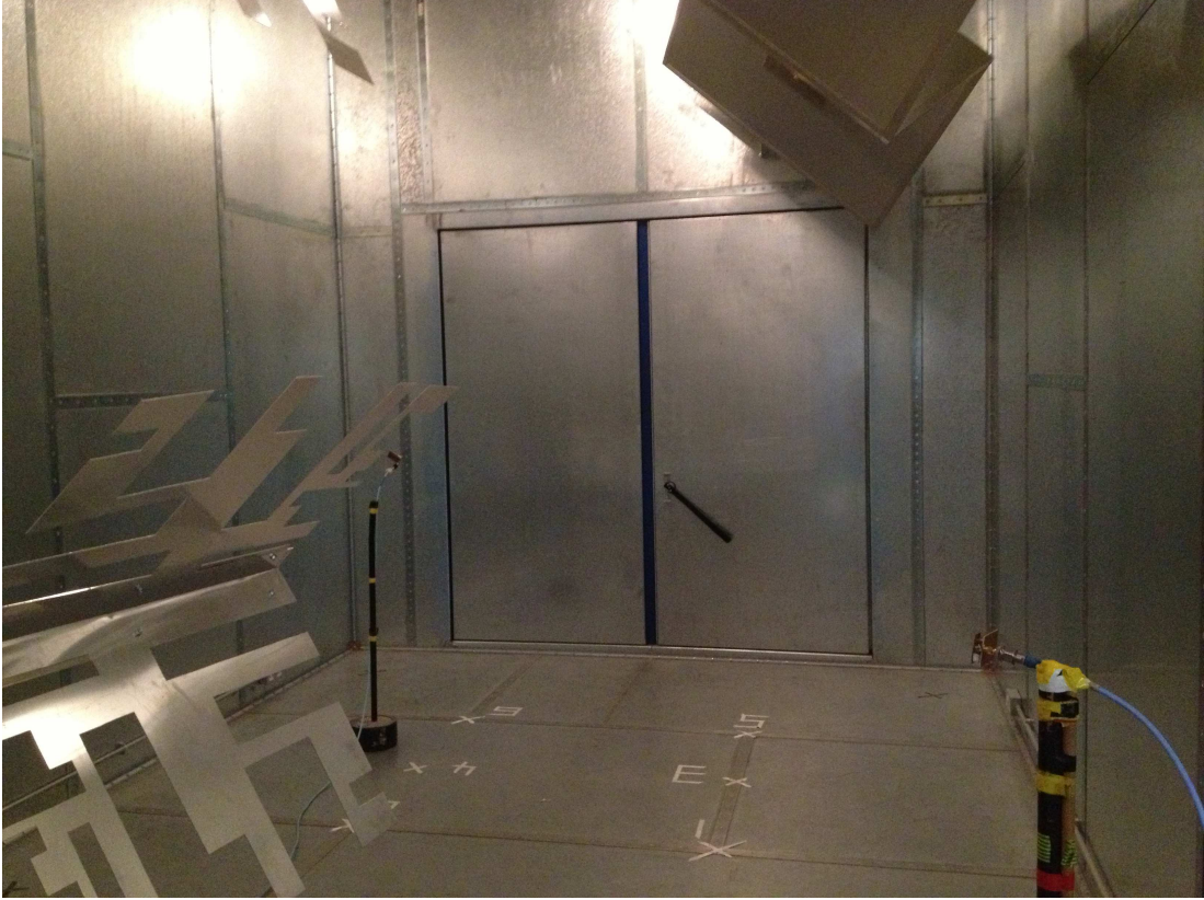
Figure 5.2: The Reverberation chamber at the University of Liverpool
