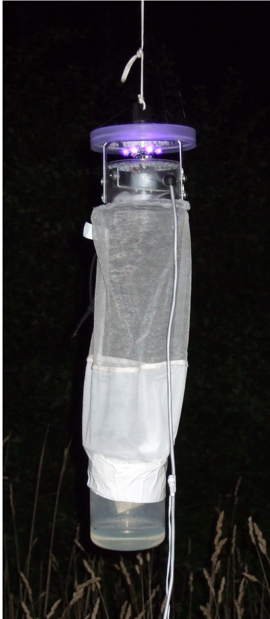
Figure 2.2: A CDC LED light-trap hanging in position. The LED lights act as an attractant to the vacuum above the fan, which collects them in the beaker below.
