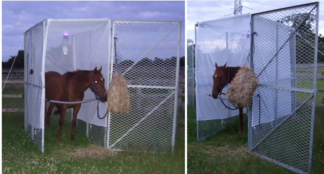
Figures 3.2 and 3.3: Experimental setup used in preliminary study two, showing a single horse within the cages. A single CDC light-trap is positioned above the horse. Netting covers the two sides, roof and part of the rear of the cage.
