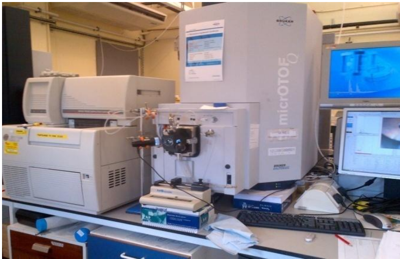
Figure 2.8 Showing the CE-MS instruments in the proteomics laboratory at Glasgow University where the proteomic experiments were performed. The CE is on the left, the MS is in the middle which is connected to the computer.
