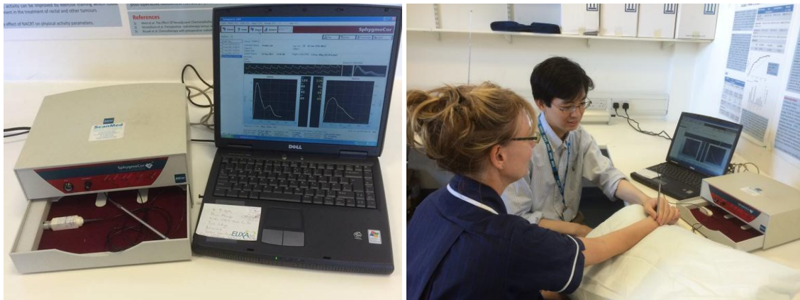
Figure 2.5 The SphygmoCor (left) and demonstration of use of the applanation tonometry at the radial artery.
