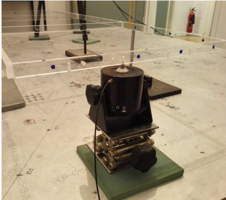
Figure 5.7 Bolt connection between shaker and beam.
