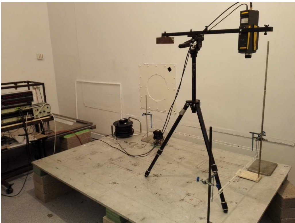
Figure 5.8 Experimental setup for measurement of Type B bending wave motion on L-junction (relevant to BT model).
