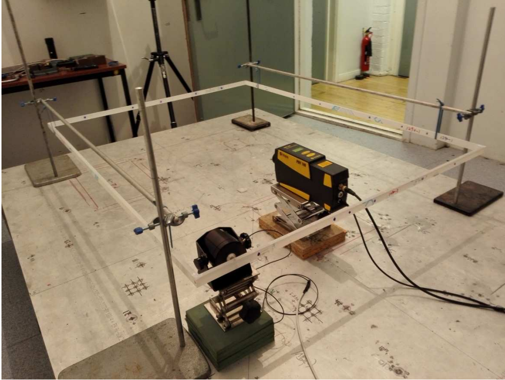
Figure 5.9 Experimental setup for measurement of Type A bending wave motion on rectangular beam frame (relevant to BL model).
