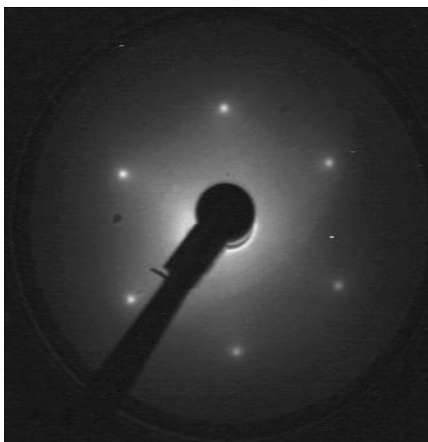
Figure 4.6: LEED image after a heavy tellurium dose no longer showing c(2\times 2) symmetry but instead hexagonal. Image taken with an electron beam energy of 70eV
