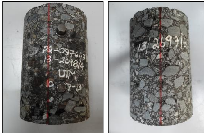
Figure 38. Examples of the specimens prepared from the field mixtures for testing.
