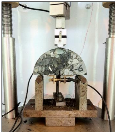
Figure 43. Set-up for monotonic SCB test.
