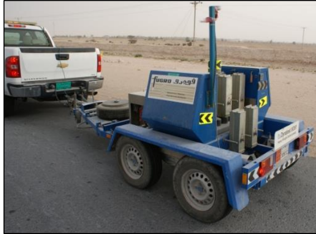
Figure 23. FWD test carried out on the trial road.
