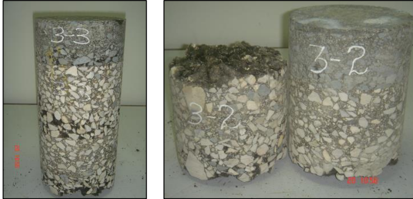
Figure 36. Segregation in the extracted field cores from trial section 3.
