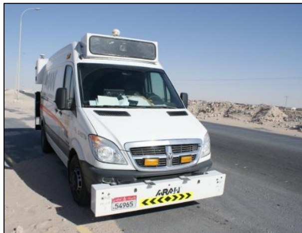
Figure 21. Automatic road analyser vehicle collecting data from the trial road.
