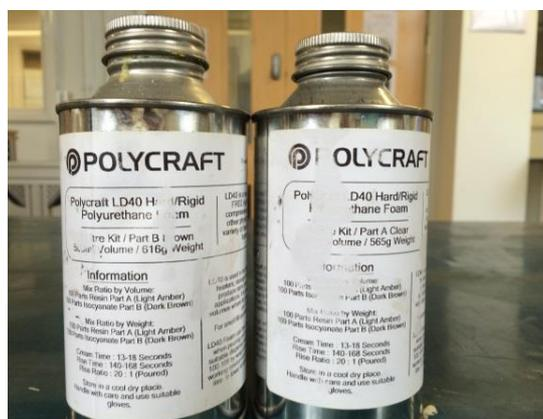
Fig. 3.9 The Polyurethanes used to make low density foam
