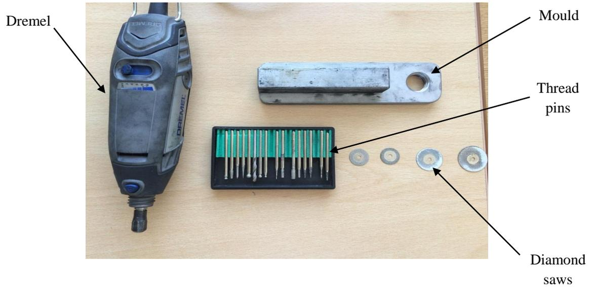
Fig. 3.1 The Dremel, saws and matched mould used to cut tubes
