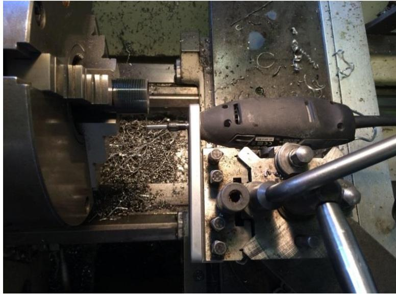
Fig. 3.3 The top view of Dremel, saws and matched mould assembled in lathe
