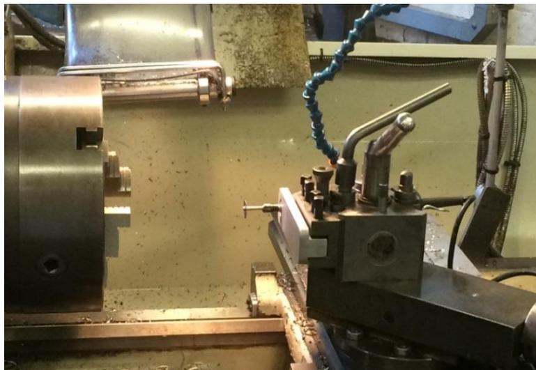
Fig. 3.2 The overview of Dremel, saw and matched mould assembled in lathe
