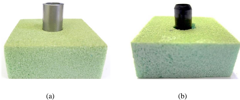
Figure 3.5 Tube partially inserted into a 50 x 50 mm P2 foam block. For clarity, the tube has not been fully inserted for (a) aluminium and (b) composite tube.
