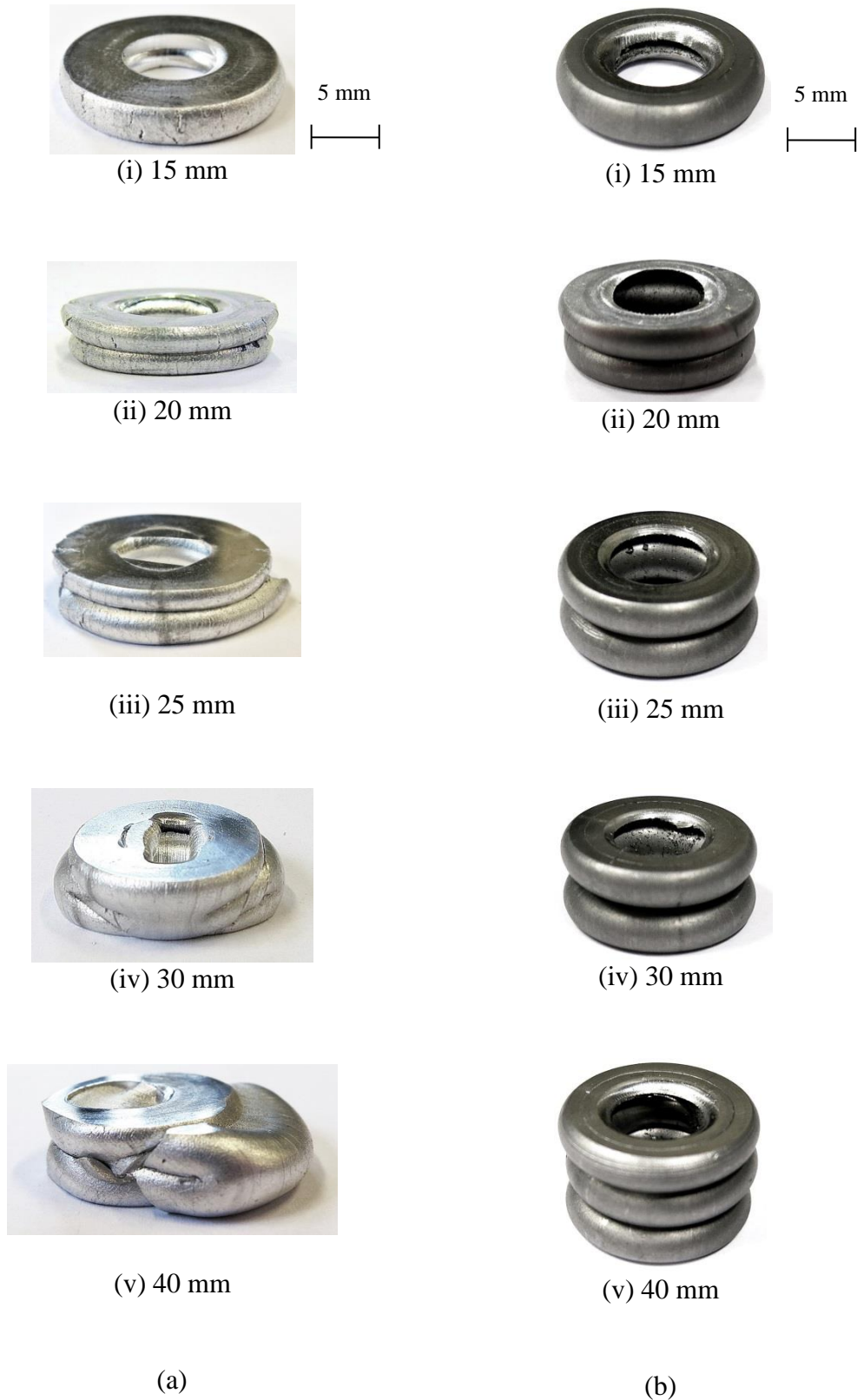
Figure 4.6 Photographs of failed samples (a) Aluminium 12.62 mm ( D/t = 5.21 ) and (b) Steel 12.62 mm ( D/t = 5.51 ). The initial tube lengths are indicated on each figure.
