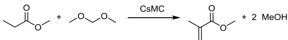
Scheme 6.6: Using dimethoxymethane as a methylene source instead of formaldehyde results in a “water-free” system for the production of methyl methacrylate.
