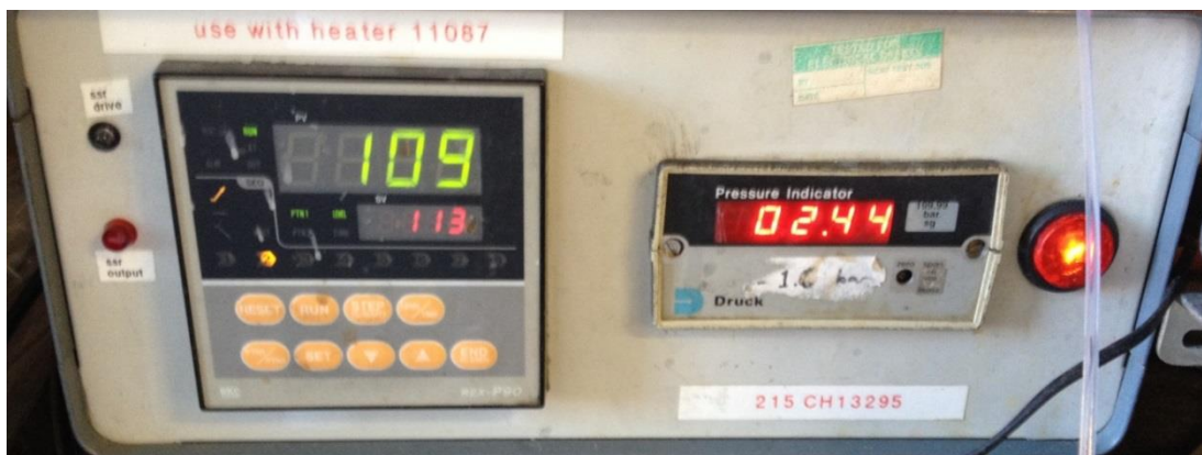
Figure 7.3: Autoclave controller before injection: Green temperature (109 °C) = temperature inside the autoclave according to the internal thermocouple; red temperature (113 °C) = desired temperature according to the heater program; pressure indicator reads 2.44 bar.
