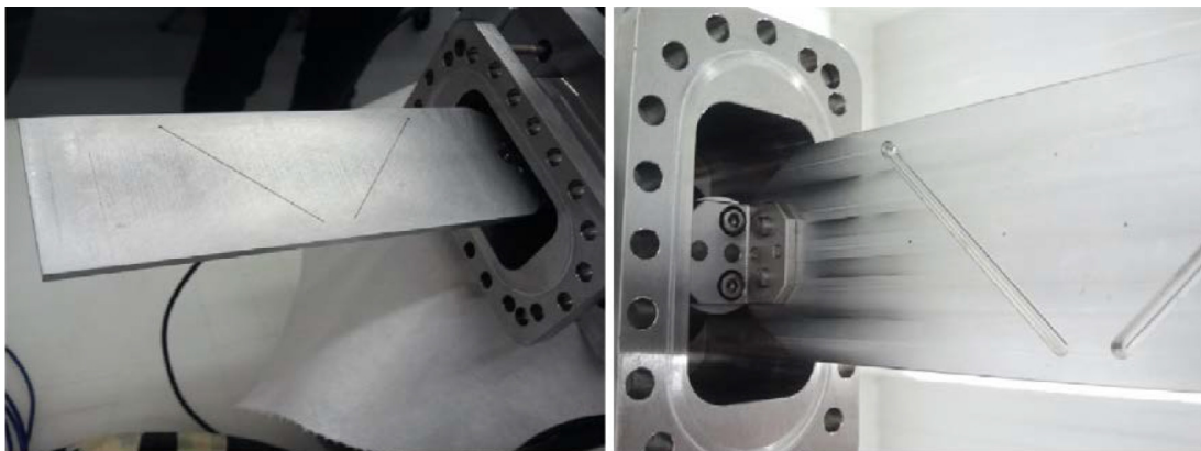
Figure 3.9: Picture of the scanning blade. Notice the almost imperceptible holes on the blade. Image taken from [81].
