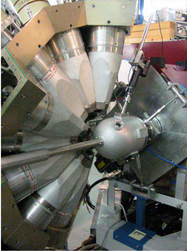
FIGURE 3.2.2: The target position of the JUROGAM detector array and the first quadrupole magnet Q_\nu of RITU. The beam pipe can be seen entering the array from the left.
