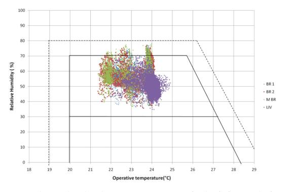
**Figure 12.** The PHV relative humidity v operative temperature comfort chart for future weather for living room (LIV), master bedroom (M BR) and the two single bedrooms (BR1 and BR2).
