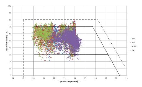
**Figure 11.** The PHV relative humidity v operative temperature comfort chart for current weather for living room (LIV), master bedroom (M BR) and the two single bedrooms (BR1 and BR2).
