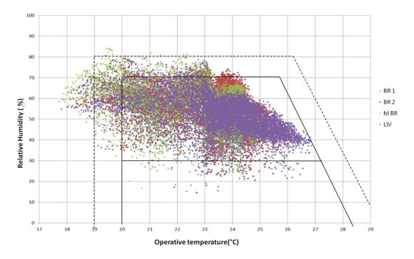
**Figure 13.** The STV relative humidity v operative temperature comfort chart for current weather for living room (LIV), master bedroom (M BR) and the two single bedrooms (BR1 and BR2).
