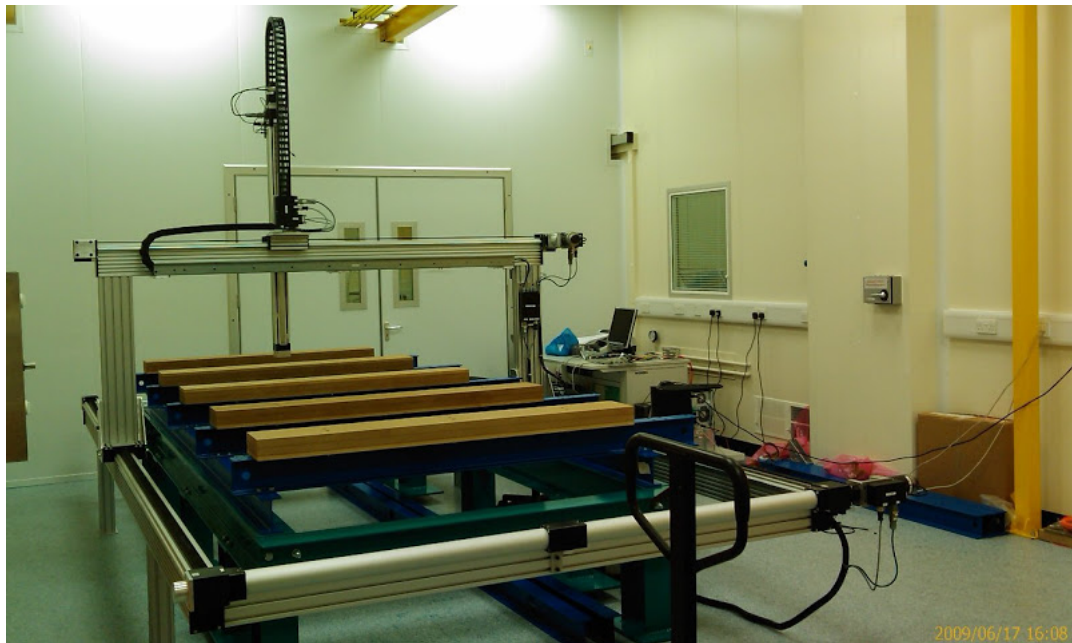
Figure 3.3: Transport frame with robotic scanning mechanism attached
