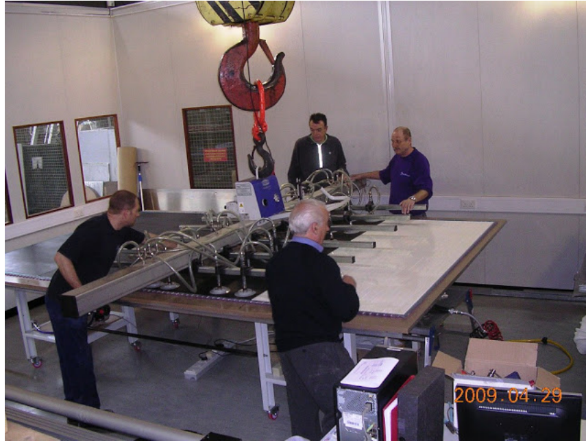
Figure 3.2: Lead layers being affixed with adhesive to plastic scintillator at Daresbury Laboratory
