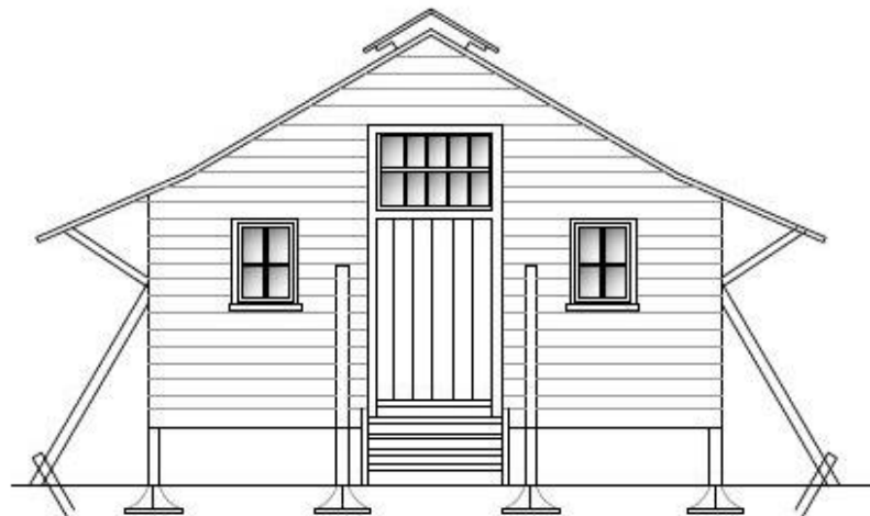
Figure 34: 1873 Hospital hut constructed for the Gold coast by Royal engineers (End elevation) 321
