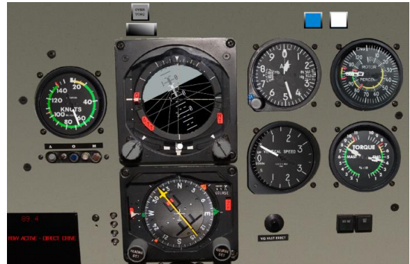
Figure 4 VAPs Bell 412 Instrument Panel
