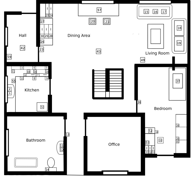
Fig. 2. A plan view of the ground floor of the University of Hertfordshire Robot House. Numbered boxes show the locations of sensors.
