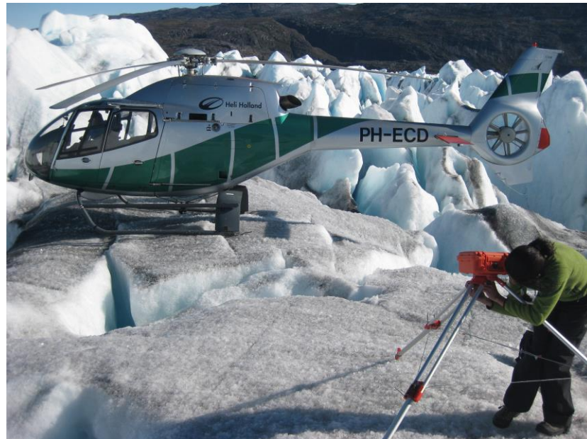
Figure 1.1 Deploying a transmitting GPS in a heavily crevassed area of the tidewater glacier Narssap Sermia, SW Greenland. The transmitting GPS allows glacier velocity to be relayed via remote satellite link for areas that are likely to become inaccessible after deployment of the instrument. (Photo: D. van As)
