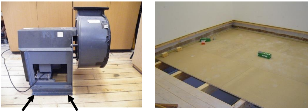
Fig. 1. Left, fan unit, free-standing in laboratory area, with two of the four contact points indicated; Right, timber joist chipboard floor under construction.
