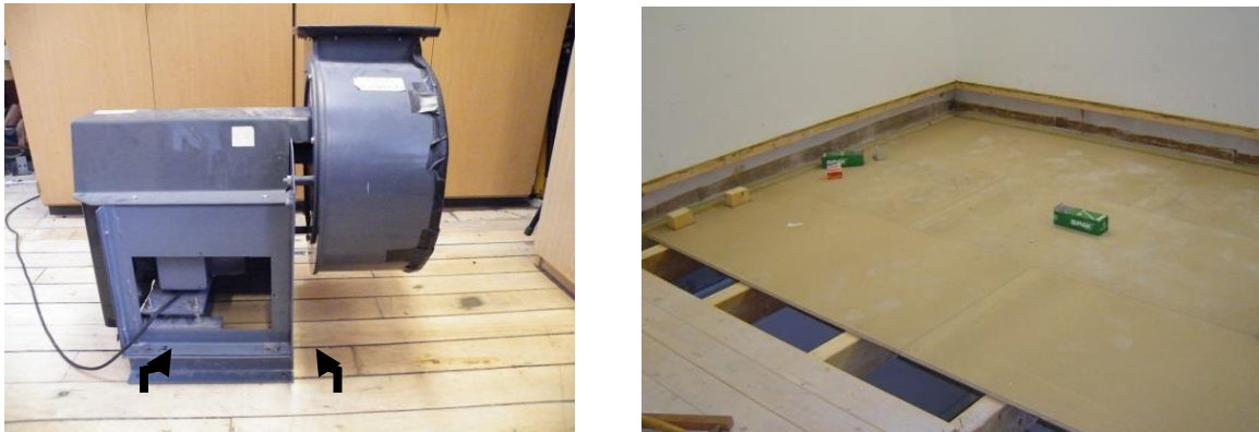
Figure 1- Left, fan unit, with two of the four contact points indicated; right, timber joist floor.
