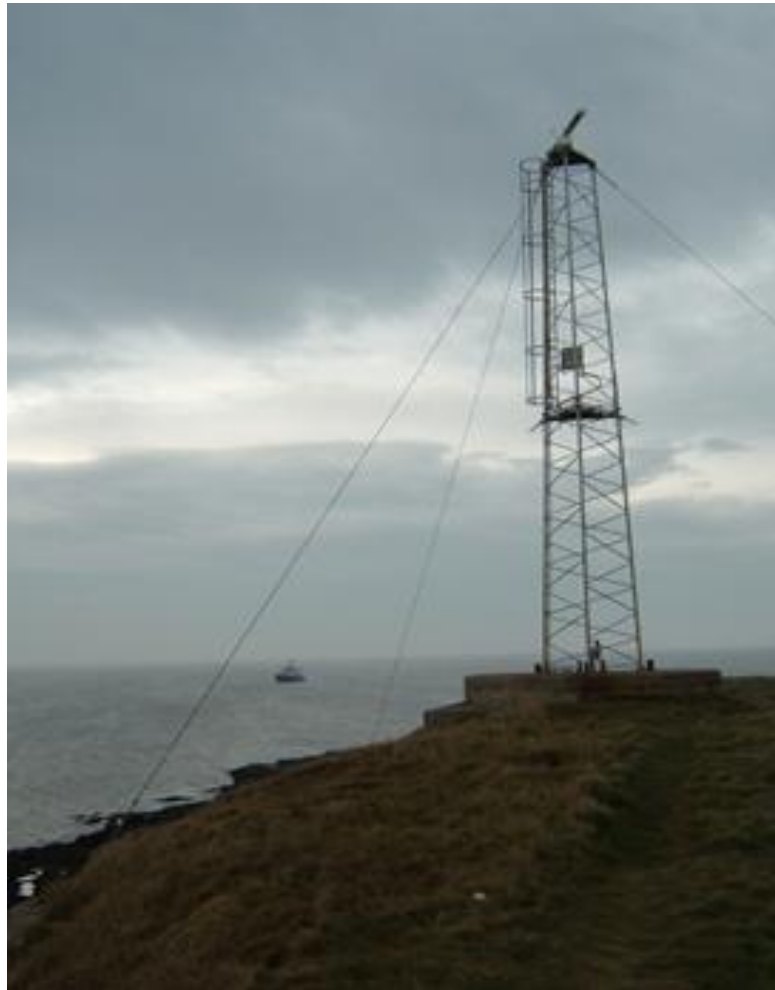
Figure 3.5: Standard X-band marine radar deployed for the purpose of gathering data used during the Irish Sea Coastal Observatory Project (COBS) during 2006 on Hilbre Island (described fully in Chapter 4).
