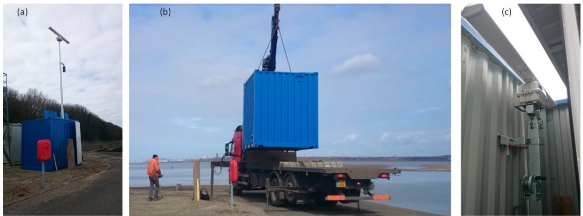
Figure 7.13: (a) Full Rapidar system deployed with mast extended to full, radar and camera system mounted, (b) Rapidar being deployed from flatbed truck, (c) Rapidar tower prior to mast extension.
