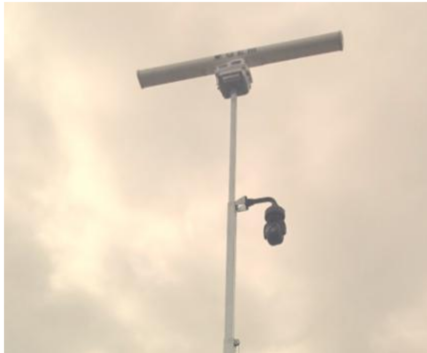
Figure 3.1: X-band marine radar manufactured by GEM Elettronica deployed at Eastham Locks, River Mersey
