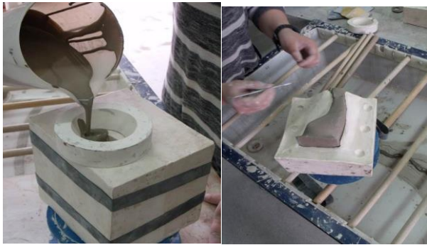
Figure 14: Slip casting the cones out of clay slip
