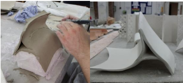
Figure 06: Forming the component out of clay slabs
