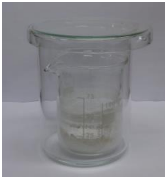
Fig. 3.7 , Two-beaker cell for salt crystallization.
