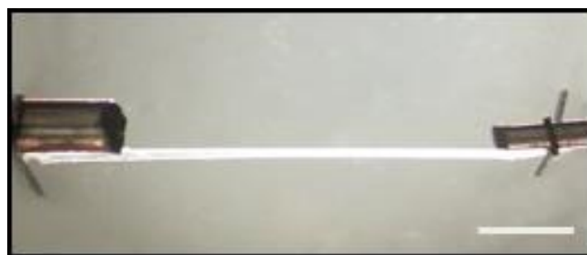
Figure 2.6 Representative image of a skinned isolated myofibre from VL muscle, attached to a force transducer and high-speed length controller. Scale bar, 400 \mu\text{m} .
