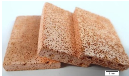
Figure 4.7: Optical micrograph showing the LCS porous Cu samples with directional porosity (40%, 50% and 60% nominal porosity from left to right).
