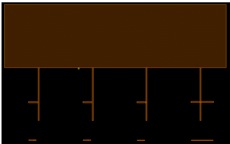
Figure 5.6-4 Etch mask shows the areas that will be removed once anodisation is complete.
