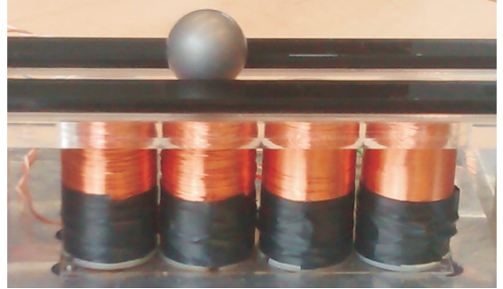
Fig. 1: Magnetic manipulation setup.
