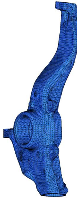
Figure 3.7. Meshes on the knuckle
