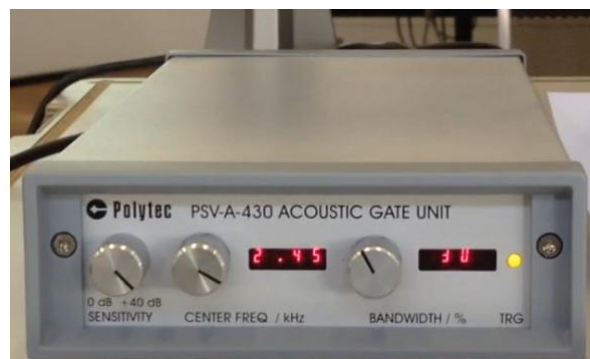
Figure 5.10. Trigger setting for the squeal test
