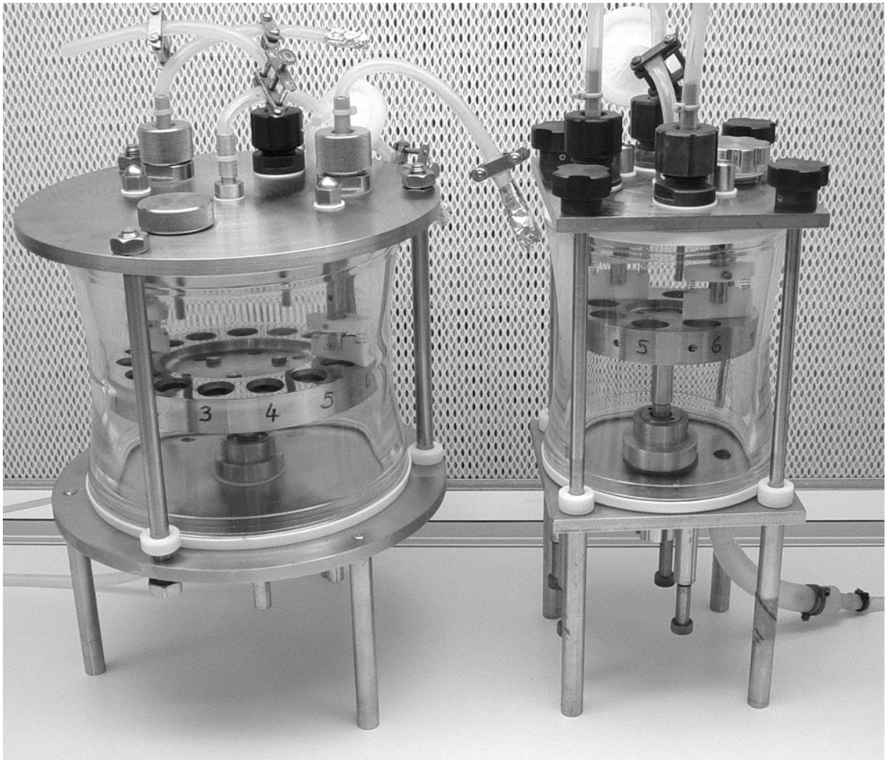
Figure 2 The 'standard' CDFF with 15 sample pans (left; University of Wales, Cardiff) compared to the compact CDFF with 8 sample pans (right; J. Abbott, West Kirby, Merseyside).
