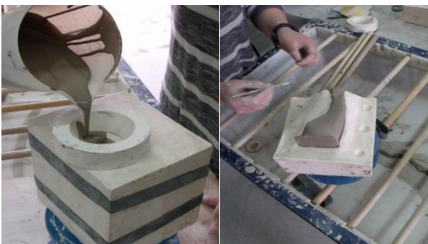
Figure 12: Slip casting the cones out of clay slip
