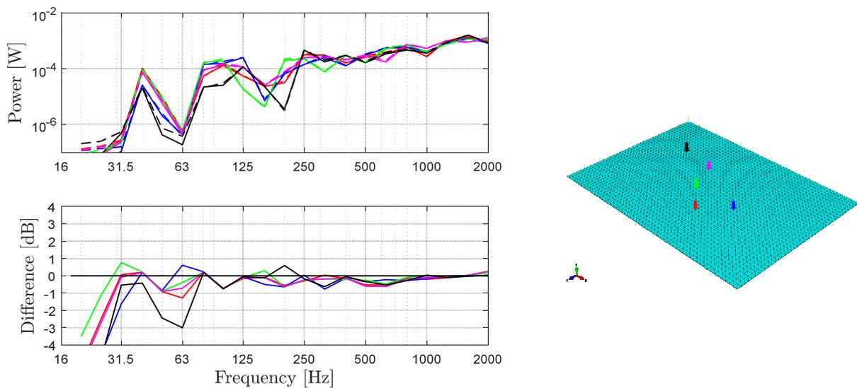
Figure 10 – FEM FFFF model: Direct injected power – solid lines, reception plate power – dashed lines (Upper graph), Direct injected power minus reception plate power (Lower graph)
