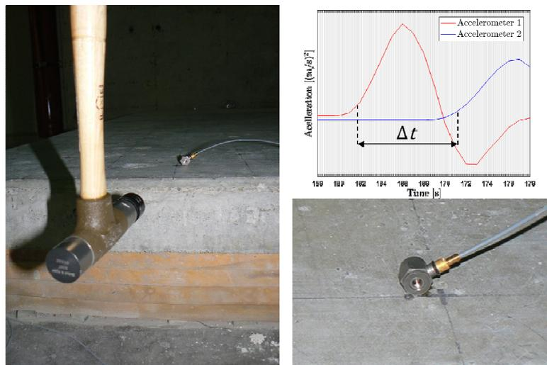
Figure 2 – Measurement setup for the quasi-longitudinal wave velocity
