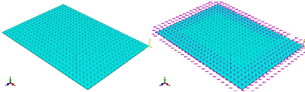
Figure 4 – FEM models: left – FEM FFFF and right – FEM Sylomer
