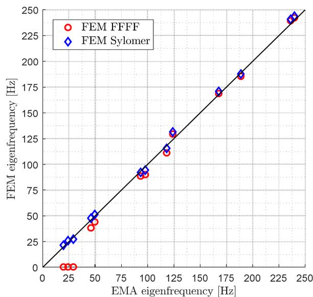
Figure 7 – Comparison of natural frequencies for corresponding mode pairs below 250Hz
