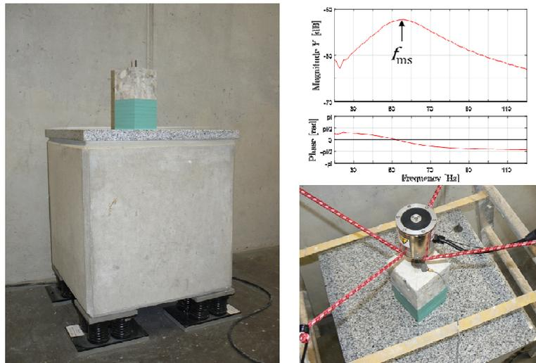
Figure 3 – Measurement setup for dynamic stiffness of the resilient material
