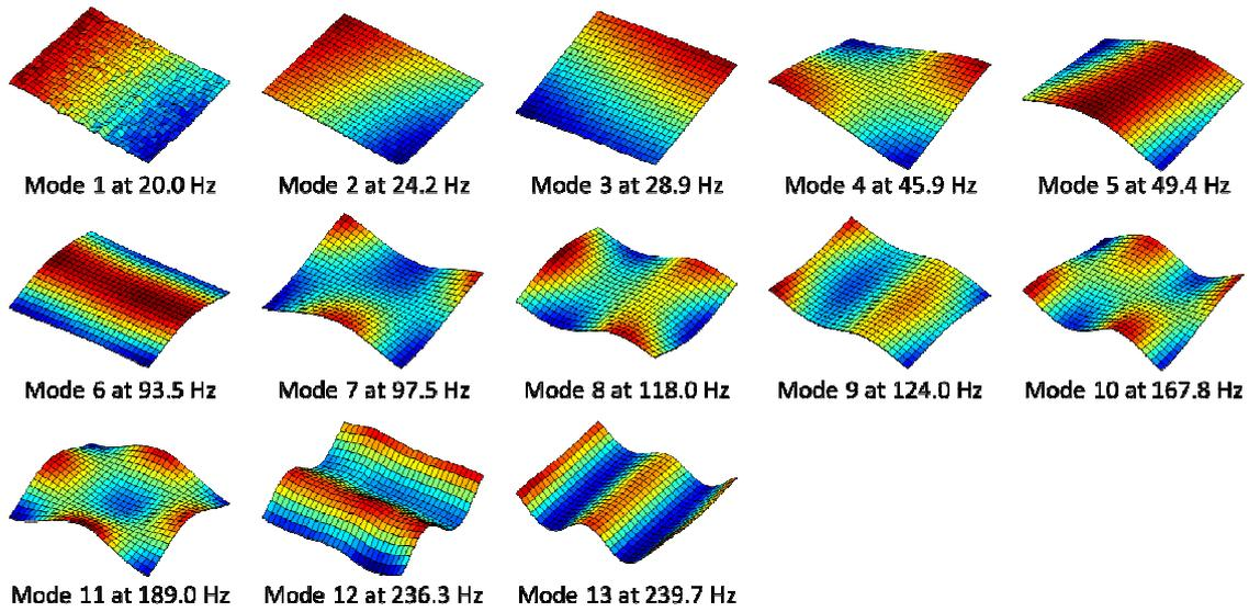
Figure 6 – Lowest 13 mode shapes and eigenfrequencies from EMA measurements on the horizontal reception plate
