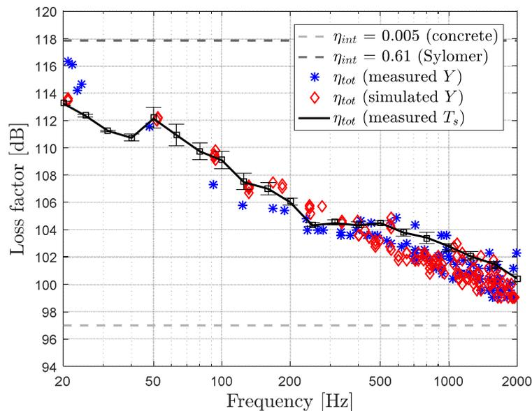
Figure 5 – FEM Sylomer model: simulated and measured loss factors
