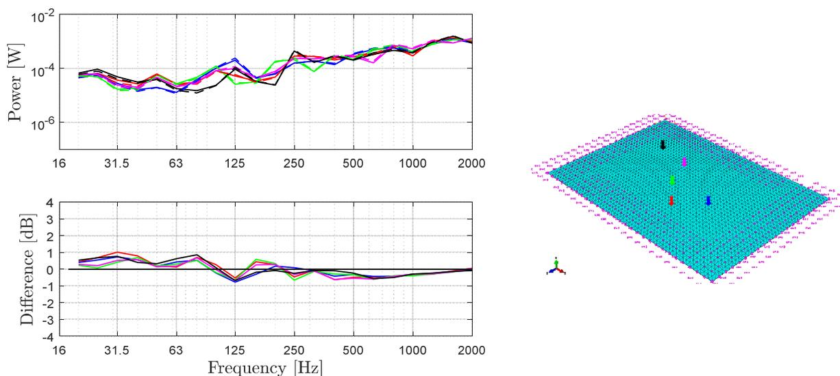
Figure 11 – FEM Sylomer model: Direct injected power – solid lines, reception plate power – dashed lines (Upper graph), Direct injected power minus reception plate power (Lower graph)
