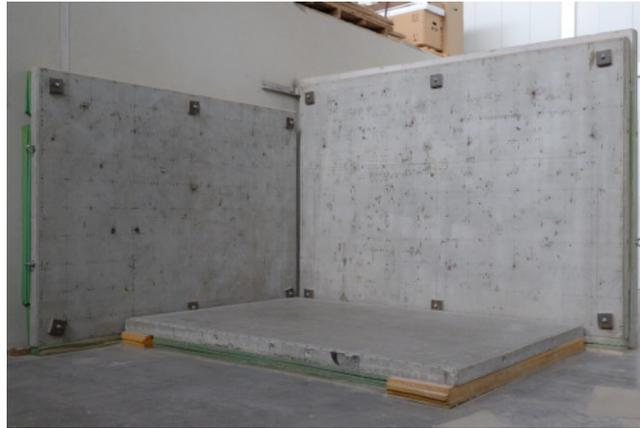
Figure 1 – Reception plate test rig at Stuttgart
