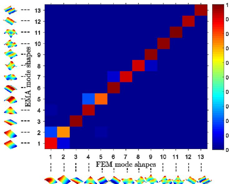
Figure 9 – MAC values (mode shapes from FEM Sylomer model and EMA)
