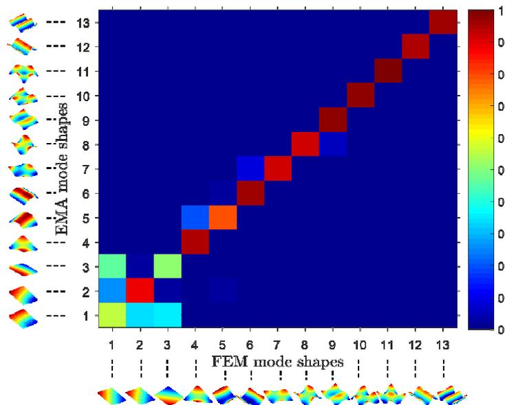
Figure 8 – MAC values (mode shapes from FEM FFFF model and EMA)
