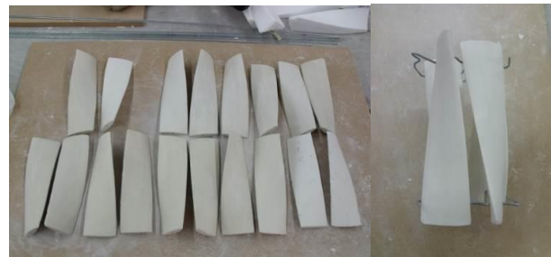
Figure 10: Formed and dried helix
