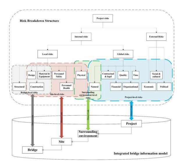
Figure 5 Basic linkage between RBS and BIM
