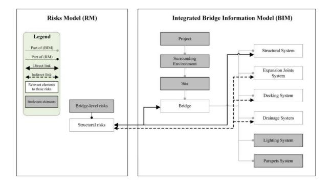
Figure 6 Linkage between structural risks and bridge information model
