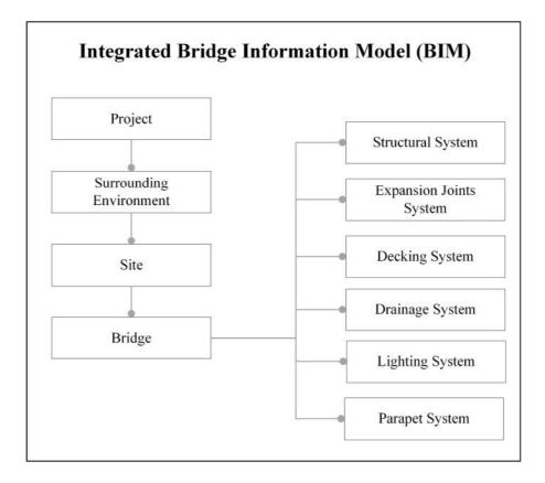
Figure 3 Separation of an integrated bridge information model
