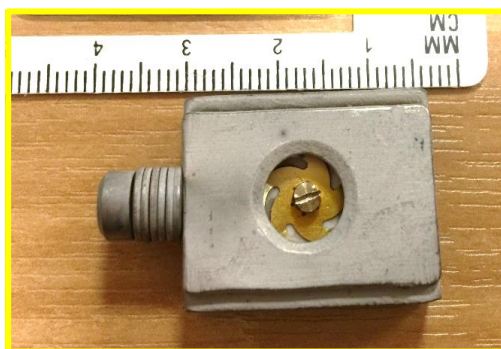
Figure 3.9: Picture of the custom made sensor head holder used in this study
